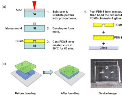
Fig. 1: Process of making the chips
