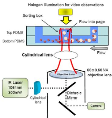
Fig. 2: Schematic of optical sorting microfluidic system with focused laser applied at the junction of the two overlapping channels
