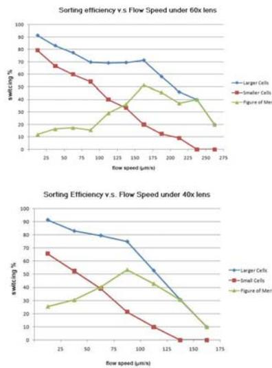
Fig. 4: Graph of sorting efficiency (%) versus flow speed (um/s)
