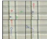
Fig. 3: Trajectories of sorted and unsorted cells produced by the device.
